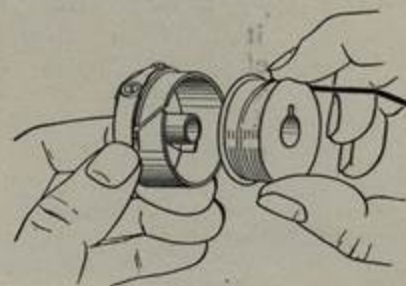
Fig. 2. After winding the bobbin, hold it between the thumb and forefinger of the right hand, the thread leading on top from the left toward the right.
